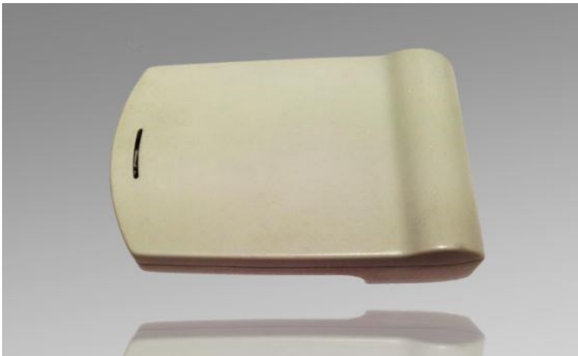
Figure 17 – A Norbit DSRC 5.8 GHz tolling tag
